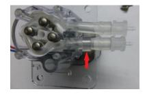
16. Secure the rotor cover [C] over the pins and then screw on the pump housing cover [D].
