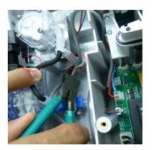
3. Remove the two tubes from the flow switch heads.
