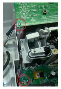
19. Screw the pump into place.
